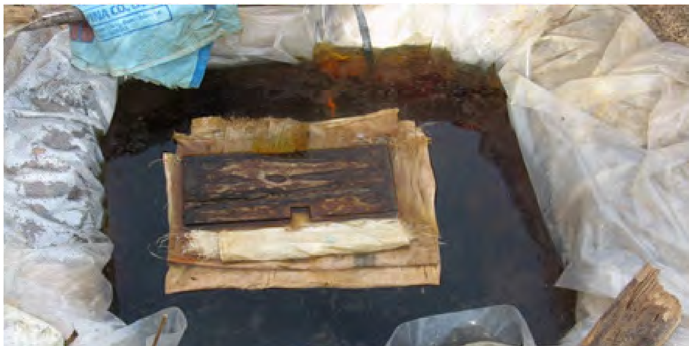
Chemical store tubs for extracting gold from ore.
